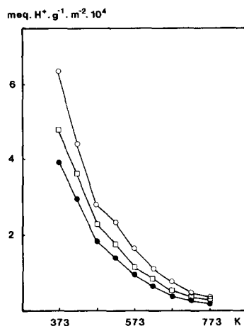
FIG. 2. Acidity distribution determined by \text{NH}_3 thermodesorption on: (○) \text{SiO}_2\text{-Al}_2\text{O}_3 24-76; (□) \text{SiO}_2\text{-Al}_2\text{O}_3 50-50; (●) \text{SiO}_2\text{-Al}_2\text{O}_3 75-25.
